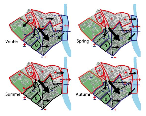
FIGURE 4.4: Seasonal heat energy potential map of St. Johann with possible energetic linkages; the arrows indicate possible heat energy streams
