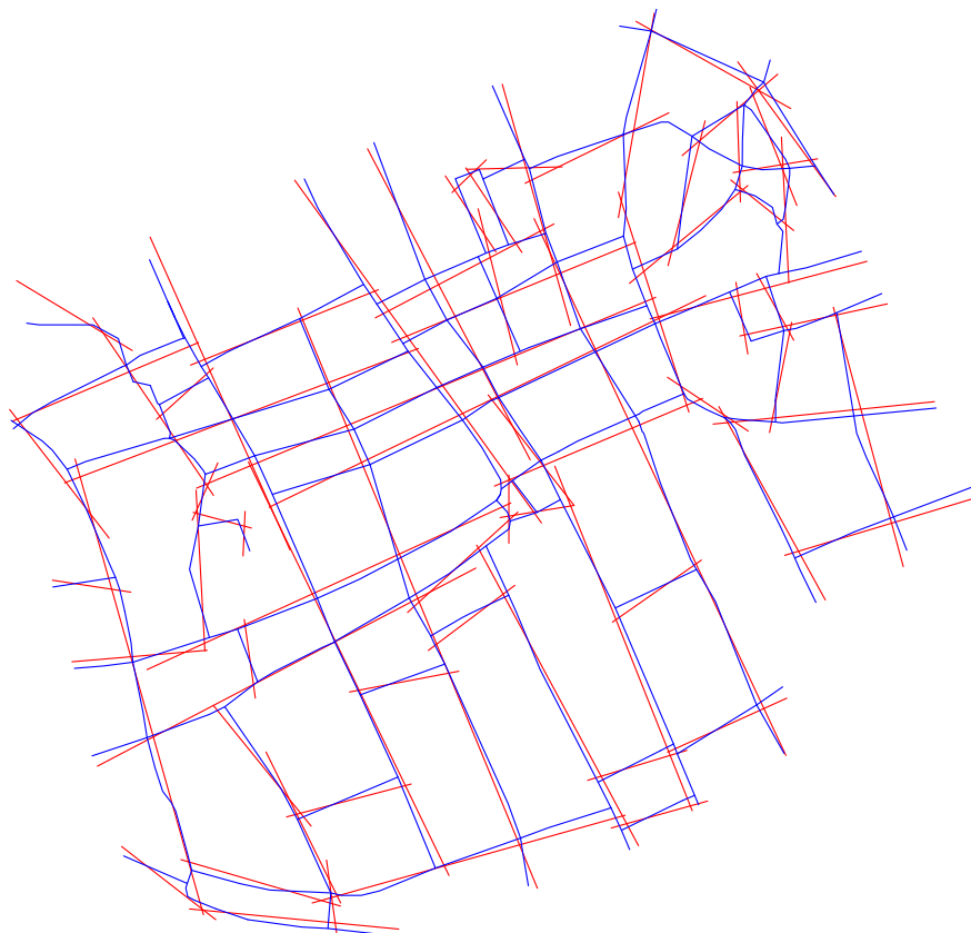
Figure 30: Inner city east inner city grid, axial map in red and road centreline map in blue
