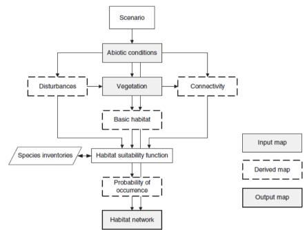
Figure 4.6 Flow charts for GIS-based predictive modelling
