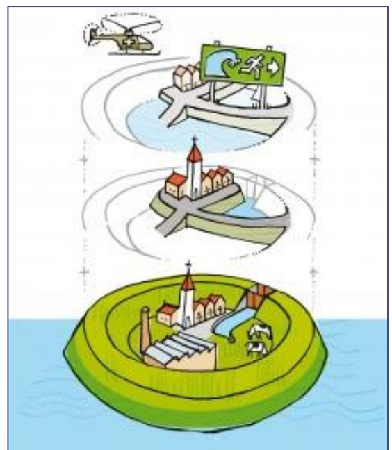
Fig. 9: Multi-layer safety, (Source: National Water plan)
