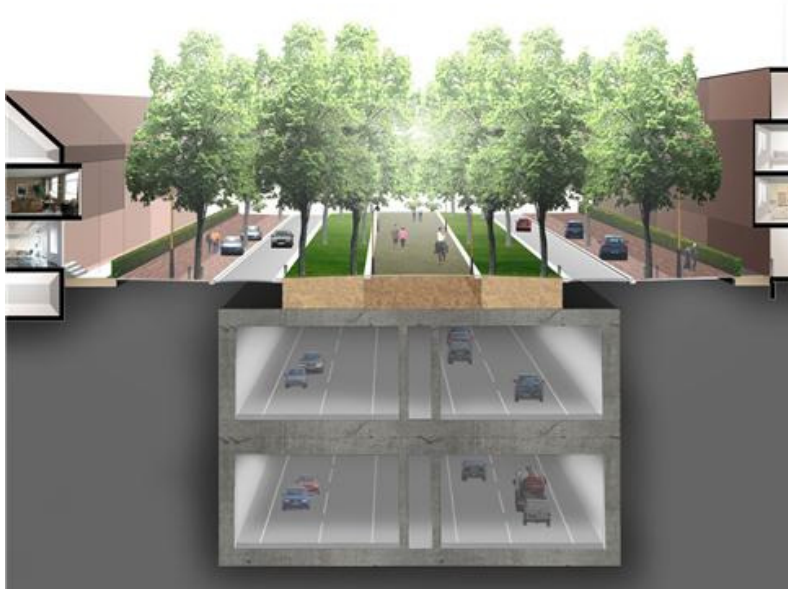
Figure 5.4 The planned solution for the A2 Maastricht problems separates the transport and living functions of the area(A2 Maastricht, 2009)
