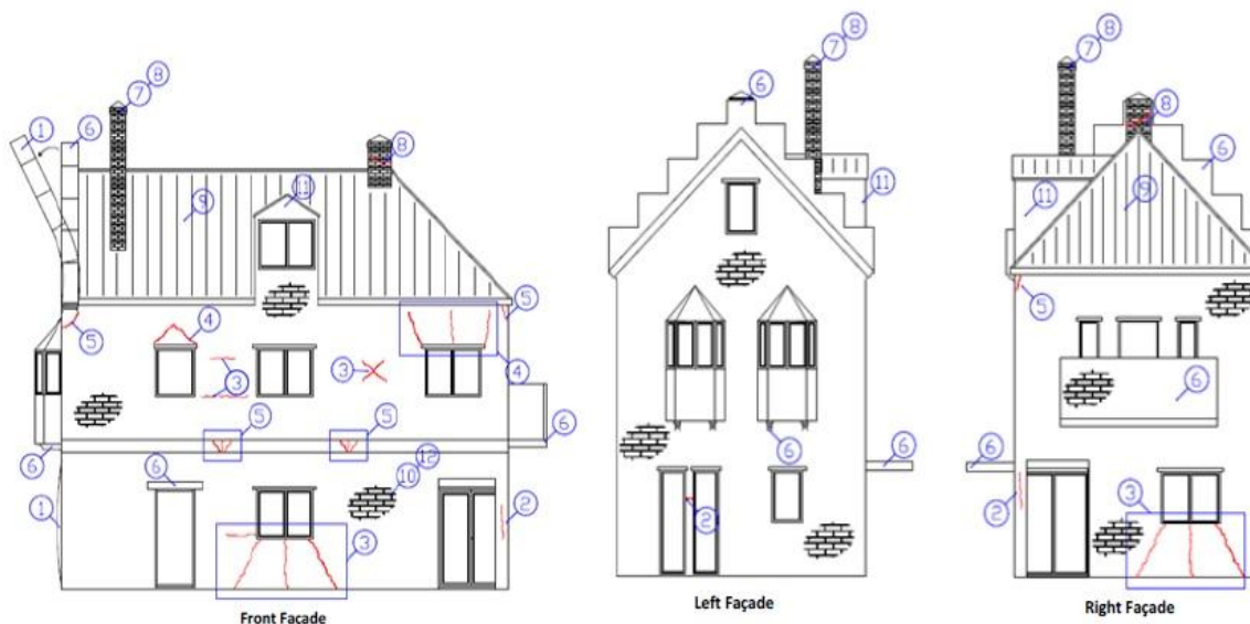
Figure 16: Overview of High Risk Building Elements (Arup, Engineering Inspection Manual EVS: Structural Upgrading, 2014)
