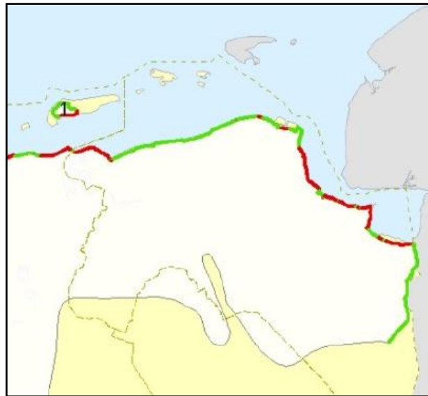
Figure 2 - Map of the levees that are approved (green) and disapproved (red) (Inspectie V&W, 2011). Scale approximately 1 : 1.000.000.
