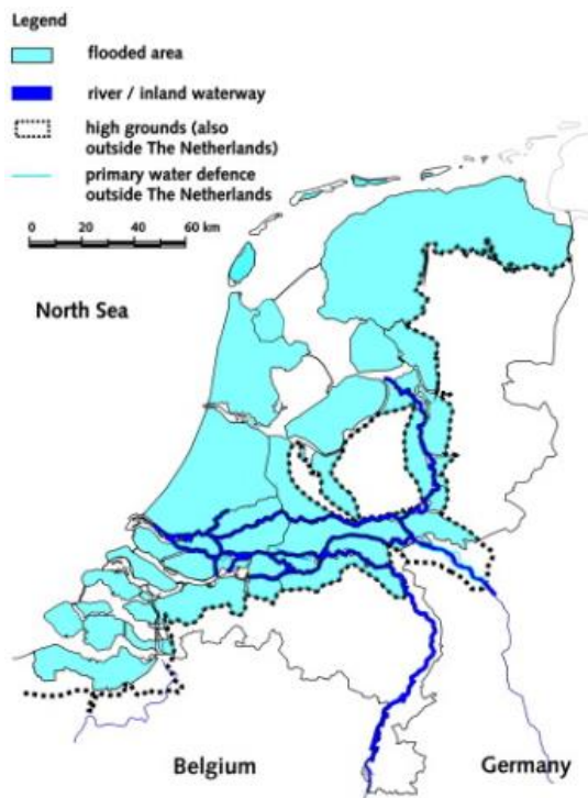
Figure 3: Currently about half of the country is below sea level and is therefore permanently threatened by flooding, if there would be no protection. Source: Bernardi et. Al. (2008)
