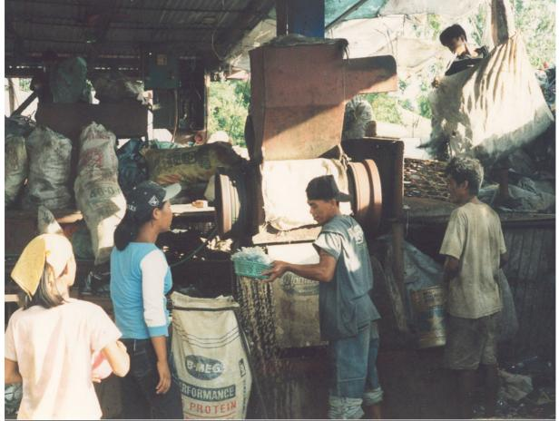
The person in the upper left corner deposits the plastics, sorted according to color and type (in the sac), through the shredder. The cullets fall into a bucket filled with water where the plastics will float. Another person scoops the
