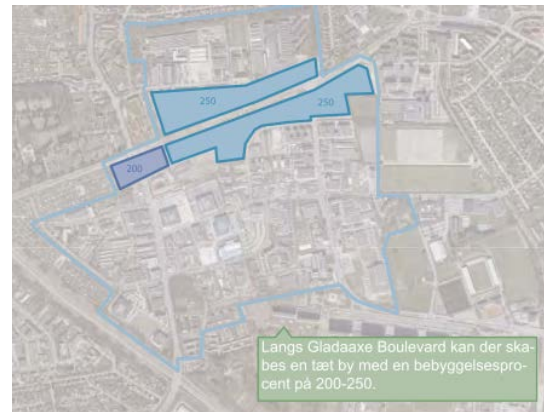
Figure 52: The application of the proximity to station principle in the Gladsaxe masterplan, showing an FSI of 200-250% (Gladsaxe Kommune, 2013)
