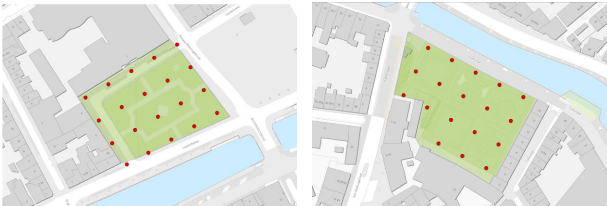
Figure 6: Systematic centric sampling grid (15x15m) applied to Guyotplein (left) and Prinsentuin (right)
