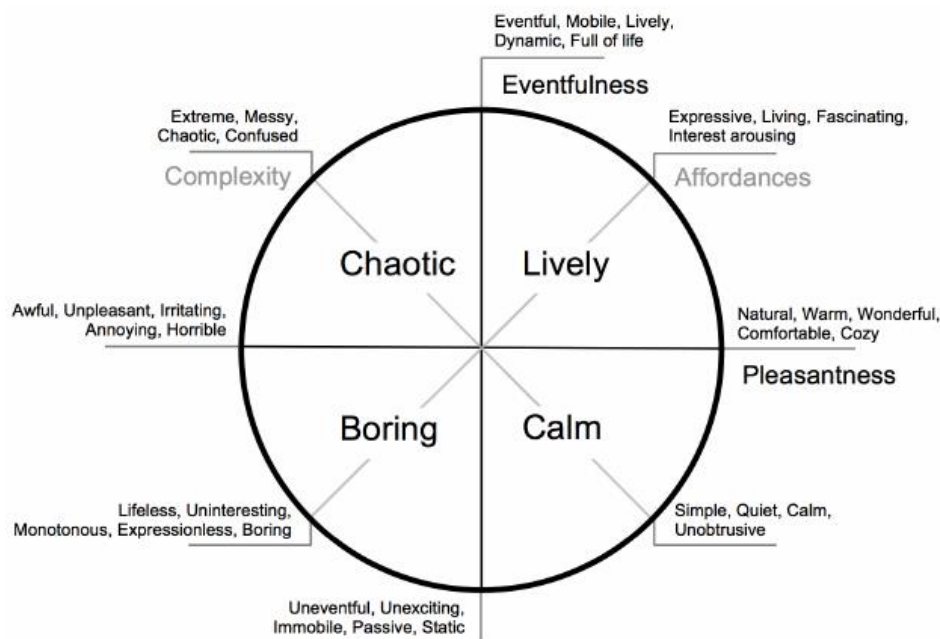
Figure 1: The Swedish Soundscape-Quality Protocol, complemented by Van den Bosch et al. (2014) depicting the four types of soundscapes (Chaotic, Lively, Boring and Calm) and their basic dimensions (Eventfulness vs. Pleasantness and Affordances vs. Complexity)
