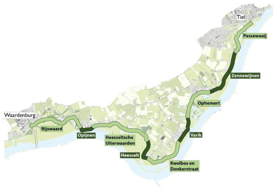
Figure 10: Tracing of the parts of the dyke to be reinforced, with accompanying village names [T2]
