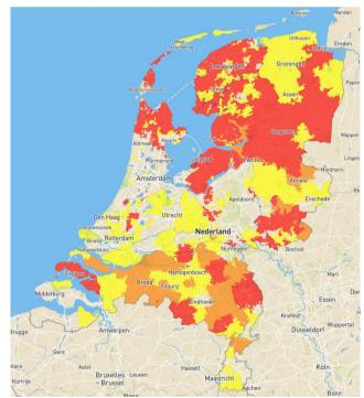
Figure 4.3: grid capacity in the Netherlands. In yellow areas, grid capacity problems are likely in the near future. Orange indicates non-structural capacity problems and red indicates no more grid capacity is left for new projects. Source: Netbeheer Nederland.
