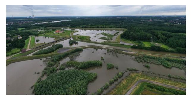
Figure 2: The Emscher-Auen, a flood retention basin in the Ruhr area, avoided downstream floods in July 2021 (Source: Wolfgang Knappmann)
