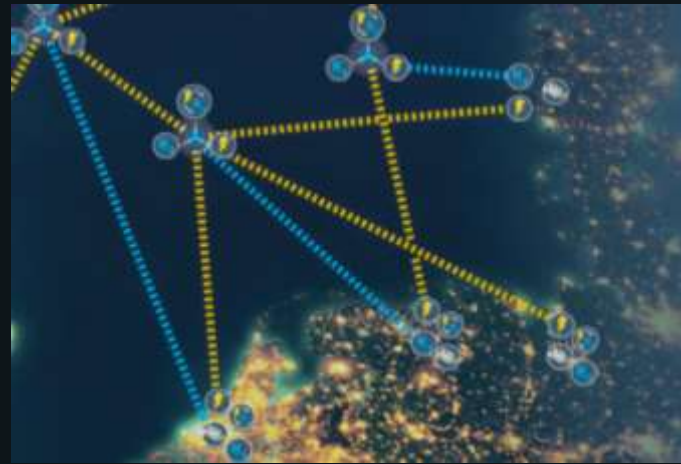
FIGURE 26. THE HUB AND SPOKE CONCEPT (THE NORTH SEA WIND POWER HUB, 2021)
