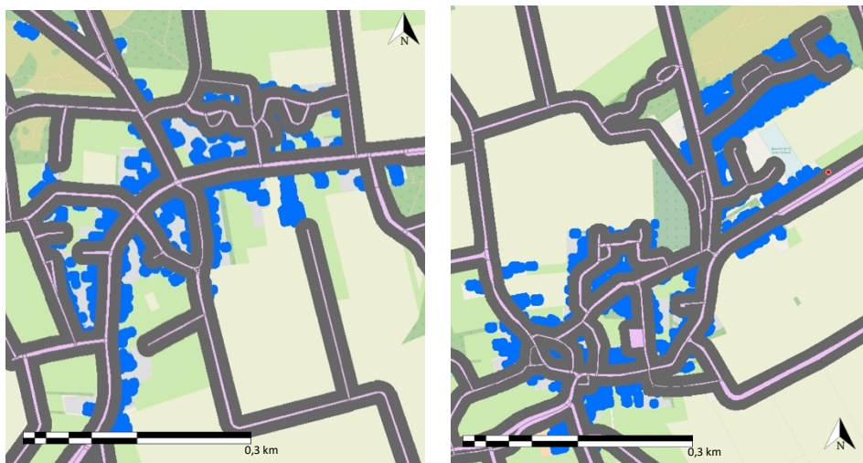
Figure 11. Not suitable safe LZ for drone to land in Gasteren (left) and Anloo (right) with buffer 25m for road and bus stop and every building for 10m.
