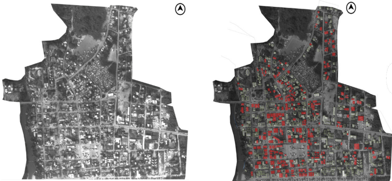
Figure 7-8: Analysis of constructions destroy by the earthquake (43%) Aerophotogrametric of before and after. Source: Astudillo J. et al. (2016) “Master Plan Canoa 2016”
