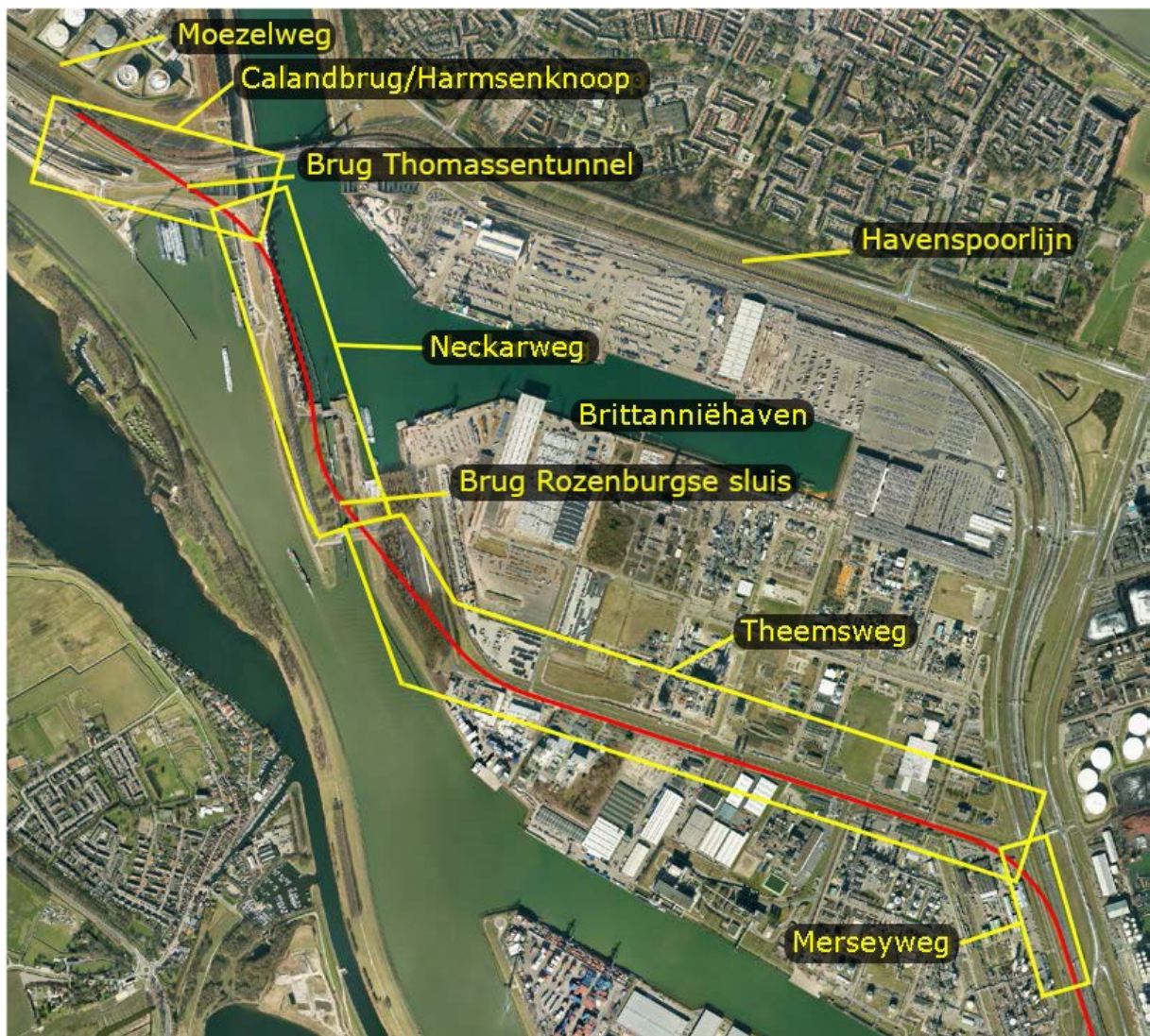
Figure 3 Map of the new route of the Havenspoorlijn line over the Theemswegtracé (red). Source: RailwaySafe BV
