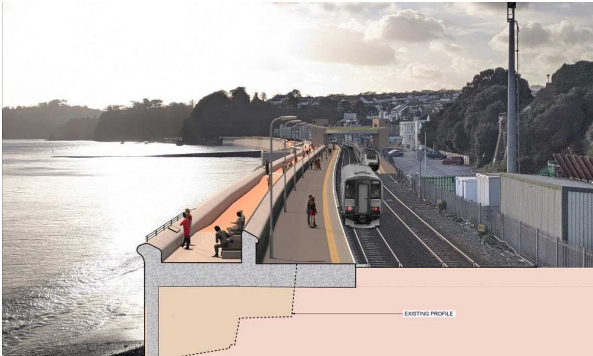
Figure 6: Artist's impression of completed phase 2 of the seawall improvement project. (Source: Network Rail)
