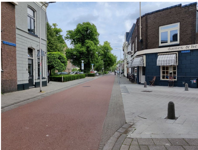
Figure 2. Bicycle street where cars are a guest and must stay behind cyclists in Assendorp, Zwolle.
