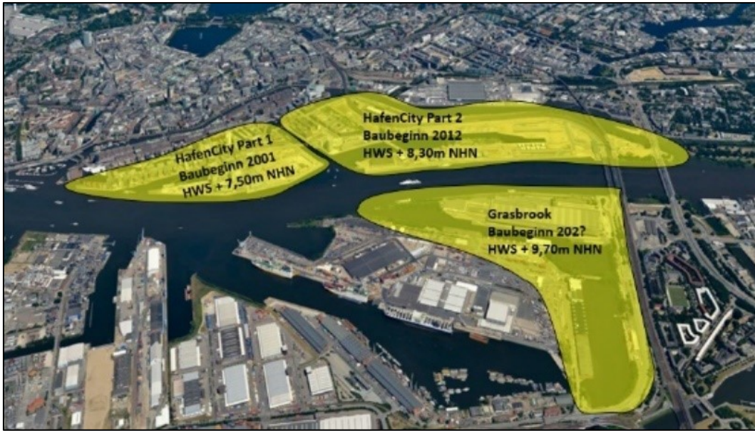
Figure 25: Comparison of the flood protection height in the HafenCity and the Grasbrook (created by the author based on GoogleMaps and information's from the interviewee 3)
