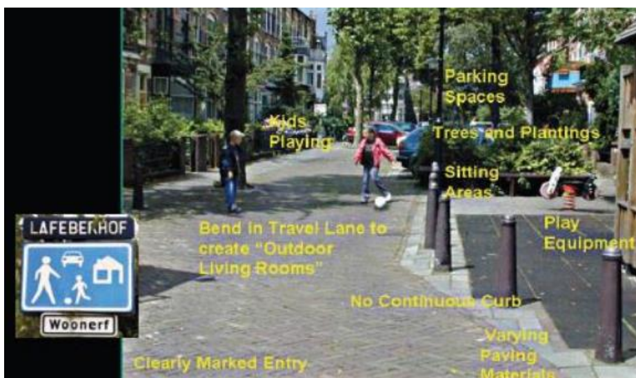
Figure 4. Five principles of a woonerf design (Appleyard and Cox, 2006).
