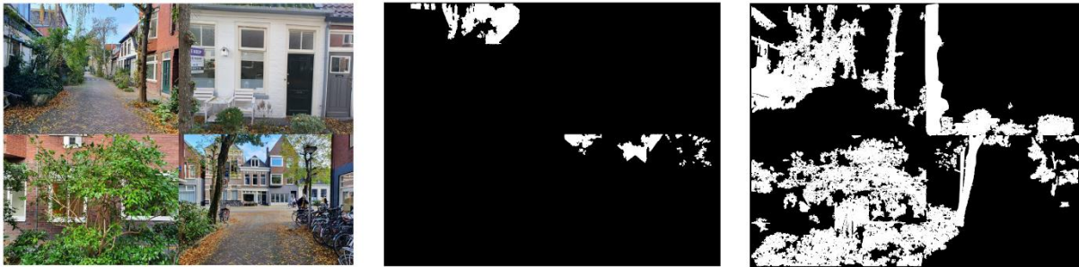
Figure 12. Example of the pixel analysis for a randomly taken picture. Four pictures laid together form the total panoramic view (left). Exclusion of sky pixels (center) and the streetscape greenery (right).
