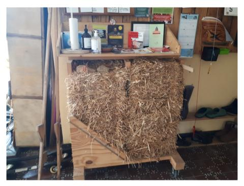
**Figure 10:** A sample of a straw building block used during the construction of the IEWAN apartment complex and showed during the monthly educative tours.
