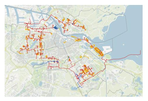
Fig. 4. In this map of the city of Amsterdam, the red lines are heat transport connections, blue lines depict cold transport, and the yellow and blue areas represent interconnected areas for heat and cold exchange. Note the near total lack of such networks in the inner city. Retrieved through the Amsterdam municipality, <u>https://maps.amsterdam.nl/stadswarmtekoude/</u>.
