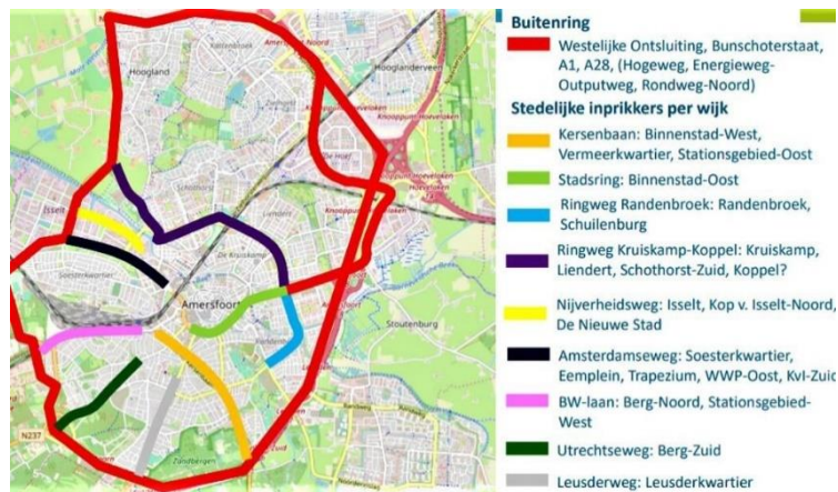
Figure 19: Traffic model of Amersfoort, showing the proposed new main ring road and the radians towards the city center (RH/DHV, 2021)
