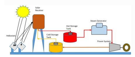
**Figure 3:** The Operation of Concentrated Solar Power Technology (Source: Albarbar and Arar, 2019).
