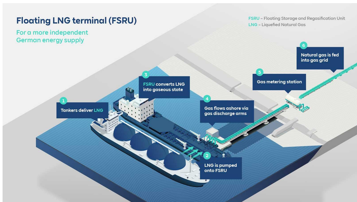
Figure 1: A tanker delivering LNG to a floating storage and regasification unit (FSRU) (RWE, n.d.)
