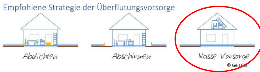
Figure 8: Strategies for flood risk precaution (in: Wunsch et al., 2023; modified by the author)
