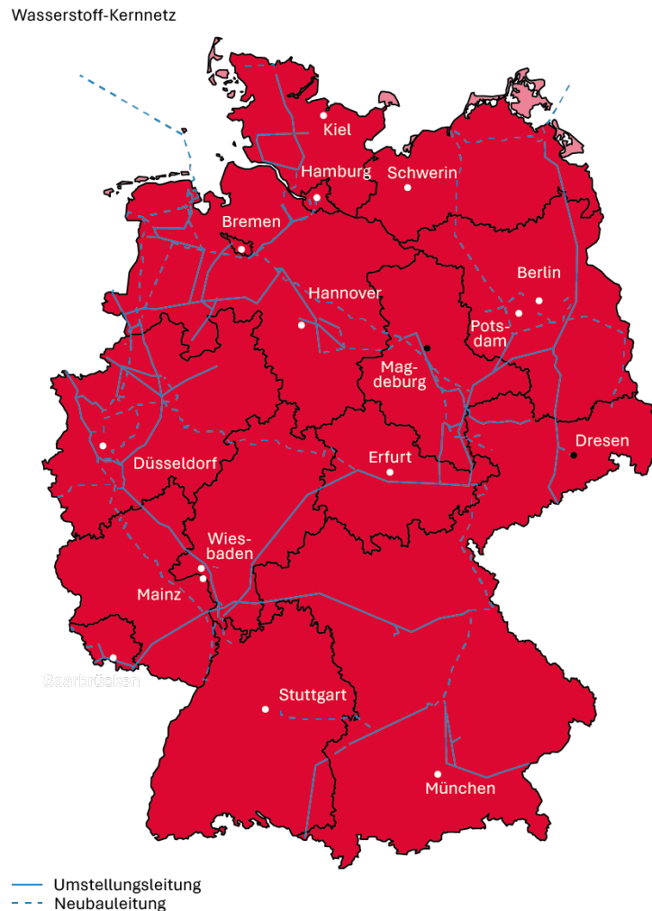
Figure 3: Map of Germany of the Federal Government's hydrogen pipeline network planning (BMWK, 2023)
