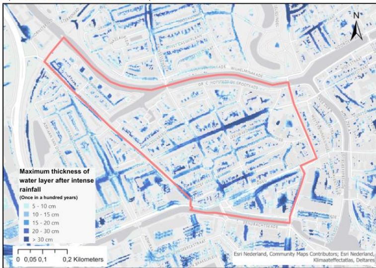
Figure 11: Maximum thickness of the water layer after intense rainfall, in the Schildersbuurt, that occurs once a hundred years (Esri Nederland et al. 2021a).
