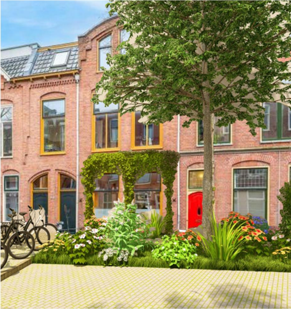
Figure 18: Impression of street design (Jozef Israëlsstraat), with wall gardens, raingardens, and permeable pavement (Stuut, 2024)
