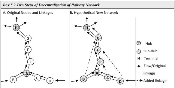
Figure 5.2 Scenario of Decentralization by Adding (Sub)hubs and Linkages
