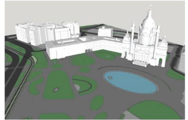
Picture 3 (current situation) Level of Detail (LOD) 3
