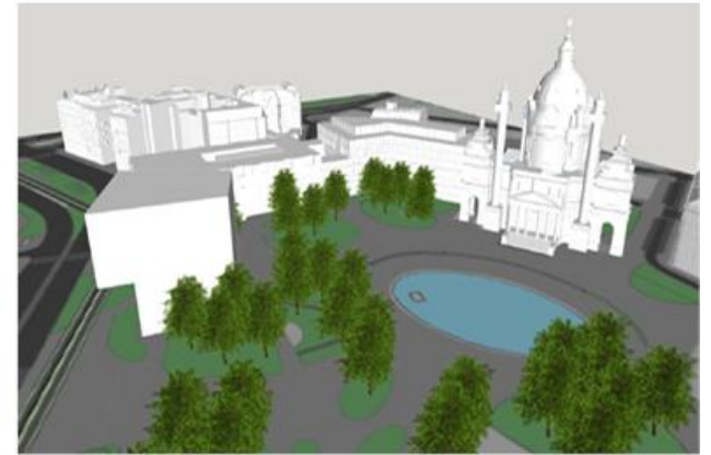
Picture 2 (possible scenario) Level of Detail (LOD) 2
