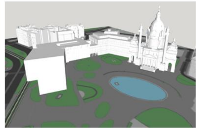
Picture 3 (possible scenario) Level of Detail (LOD) 3
