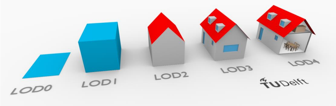
Figure 3: Varying Levels of Details in 3D urban planning models according to CityGML (TU Delft, 2016)
