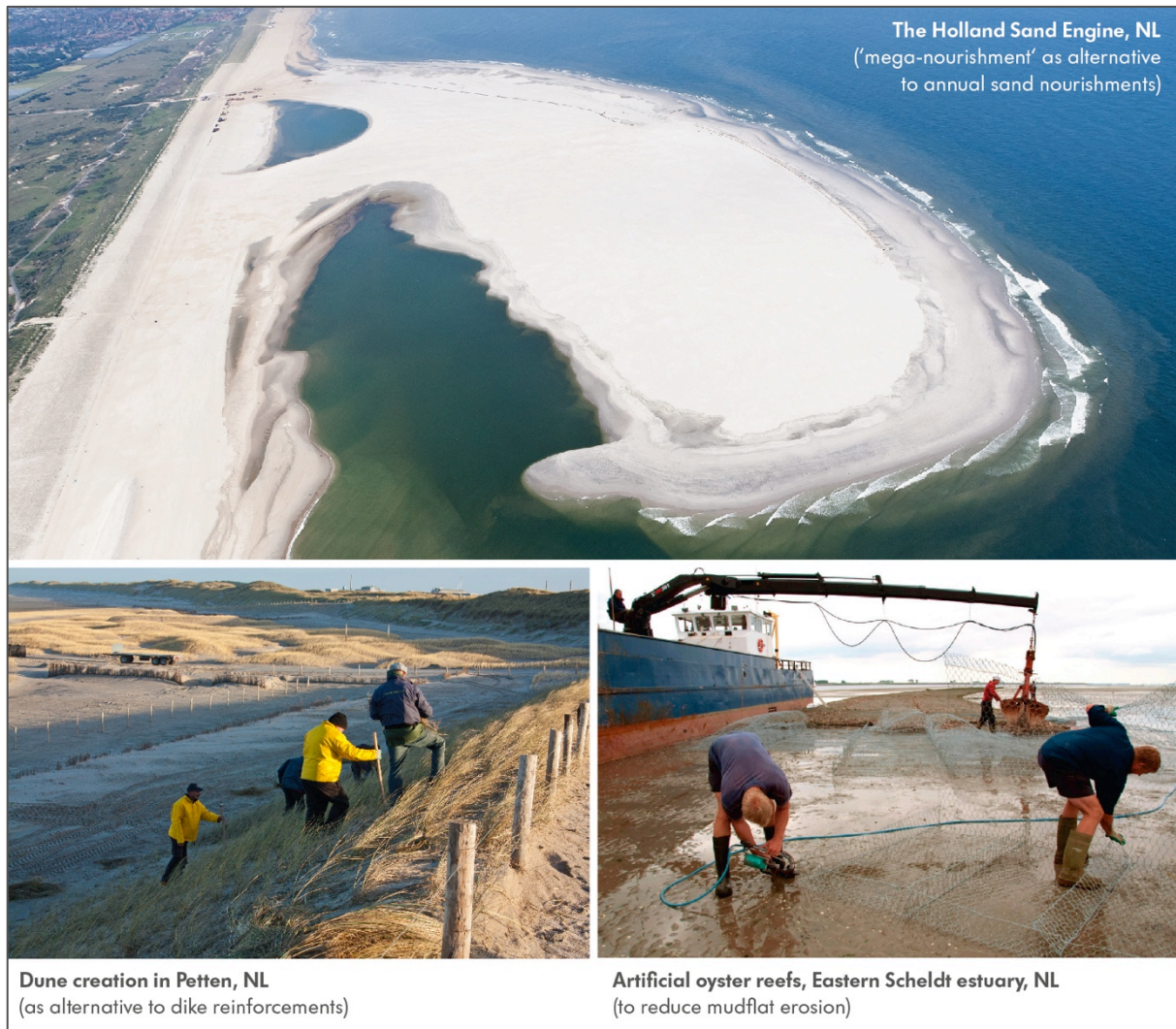
Figure 12: BwN project examples (above: Ecoshape, 2016, left: M. Martens, 2016, right: de Vriend et al., 2014).
