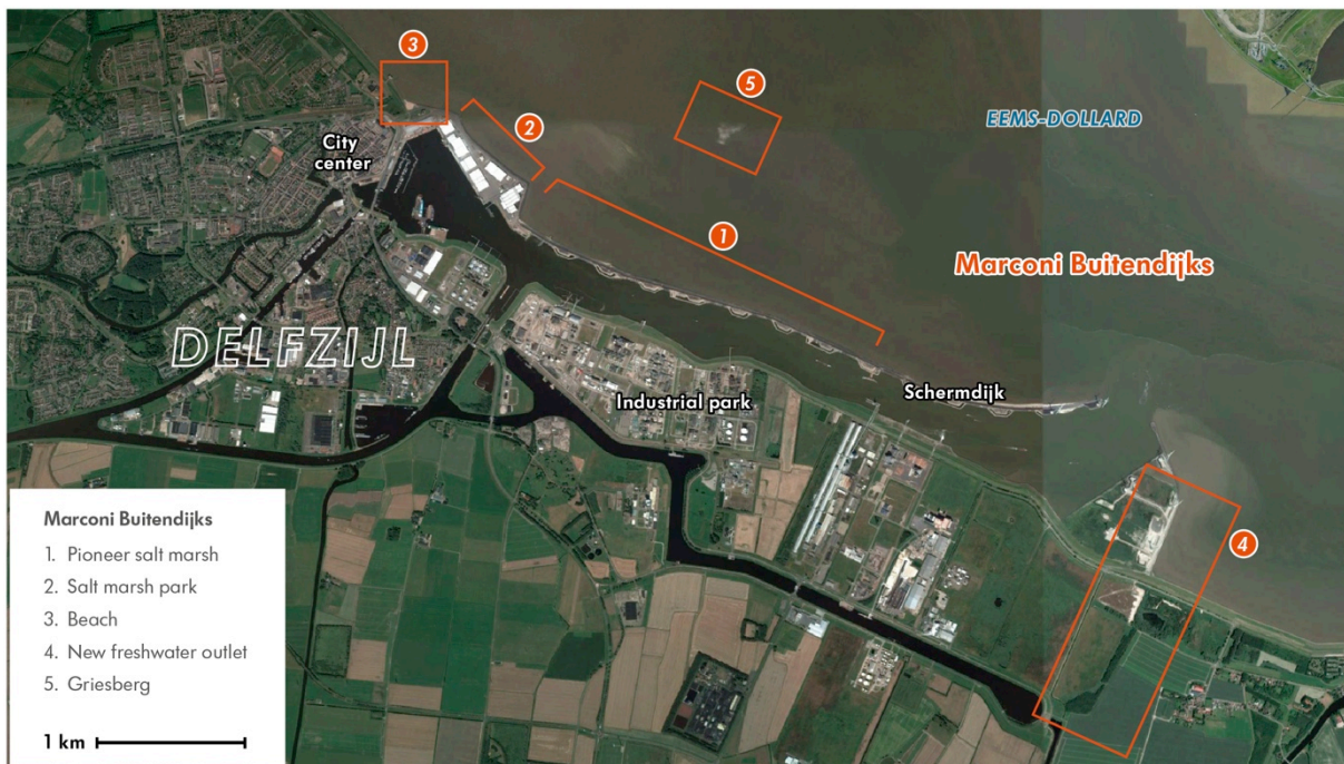
Figure 21: Aerial photo of Delfzijl showing the locations of the Marconi Buitendijks sub-projects along the waterfront (adapted from Google Earth).
