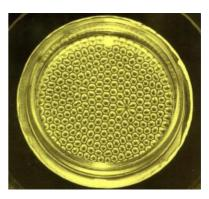
Figure II. 1. Hexagonal patterns produced in Benard's experiment (source: http://metahistory.org)
