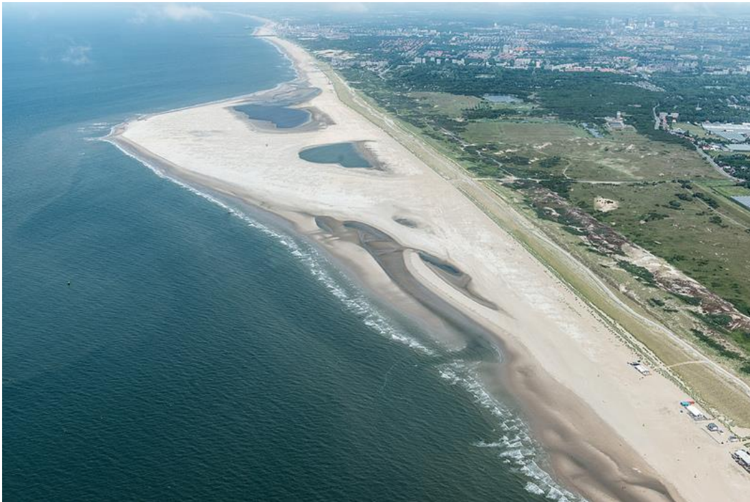
Fig. 3-5 Aerial photograph of the Sand Engine near the town of Kijkduin at 1 st of July 2013 looking northwards. The hook, which was initially open to the North closed in late 2011, due to significant morphological changes (picture copyright: Rijkswaterstaat / Joop van Houdt).
