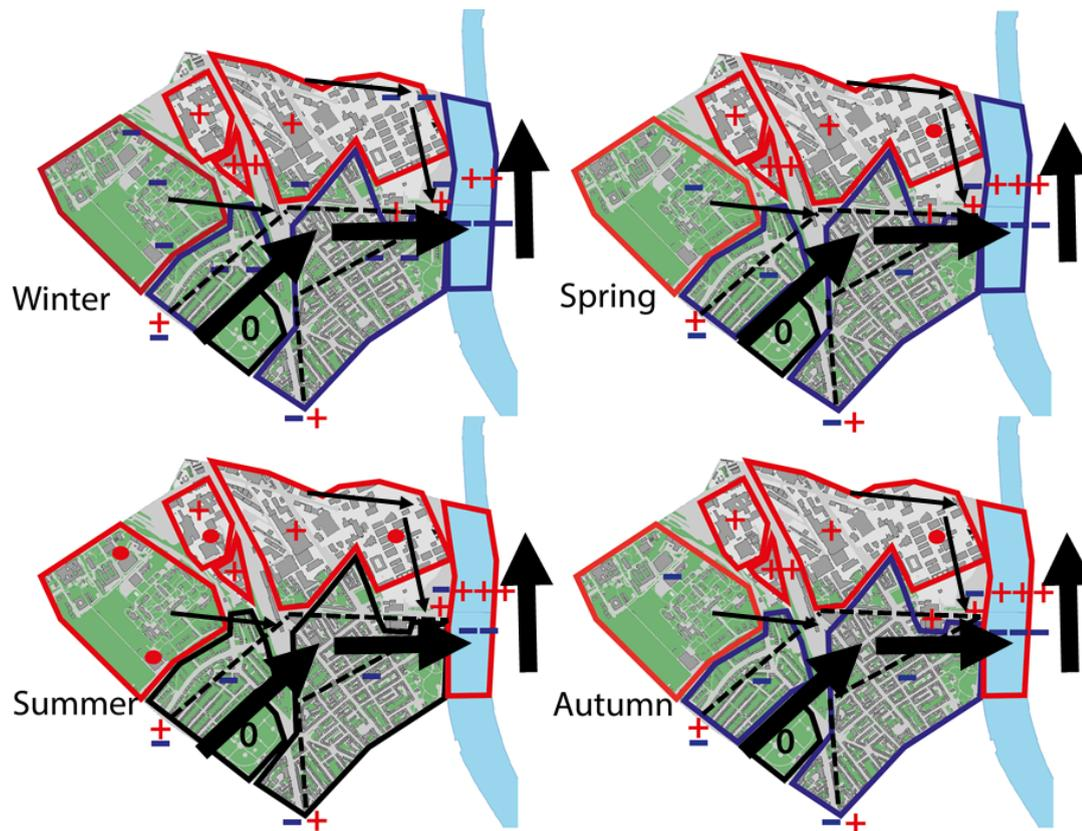
FIGURE 4.5: Seasonal heat energy potential map of St. Johann with demand and sources of heat energy, and flows of water bodies; the arrows indicate the flow direction of water
