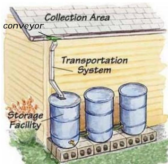
**Figure 2.1 Illustration of rainwater harvesting method**
