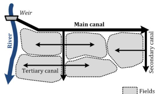
Figure 1 - Physical levels of irrigation systems
