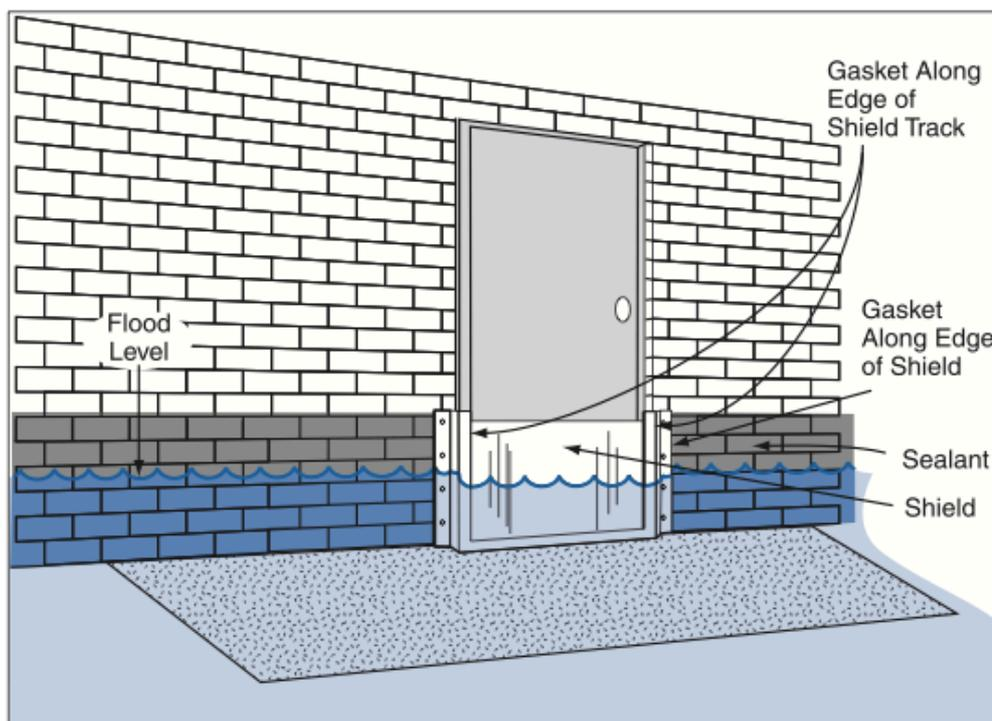
Fig. 2.07: Dry proofing of buildings, example of the wall and door (FEMA 2009)
