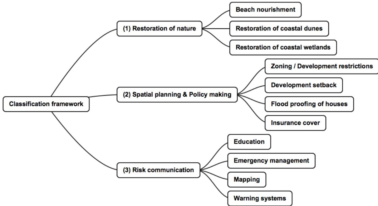
Fig. 2.14: Classification framework of non-structural measures to mitigate coastal flooding
