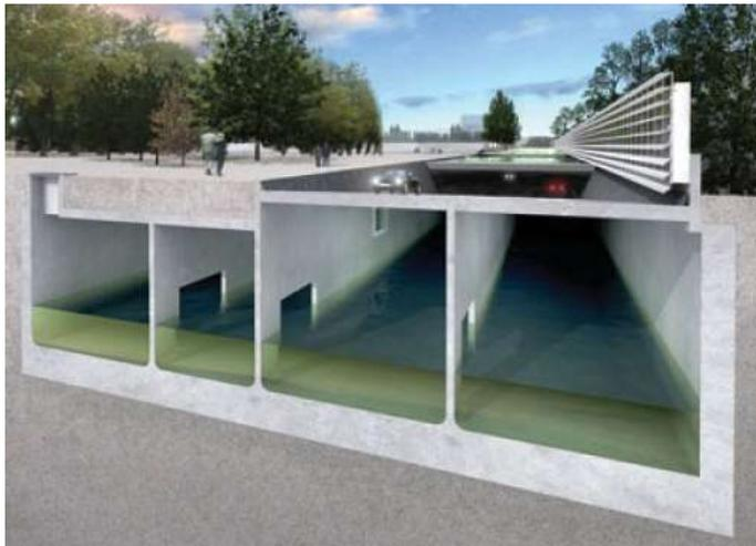
Fig. 7 Temporary excess water in underground car parks (from waterworld.com online)
