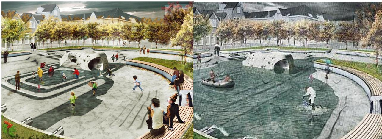
Figure 4.4: The left picture shows the empty water square and the right picture shows the water square serving as a retention area.
