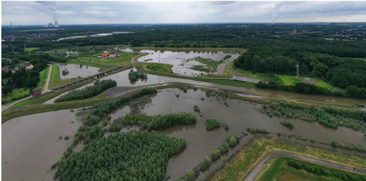
*Figure 2: The Emscher-Auen, a flood retention basin in the Ruhr area, avoided downstream floods in July 2021 (Source: Wolfgang Knappmann)*
