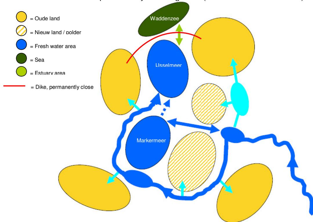
Figure 3.10 The Freshwater Scenario for the year 2100, Closing the connection between IJsselmeer and Wadden Sea, stream water using pumps
