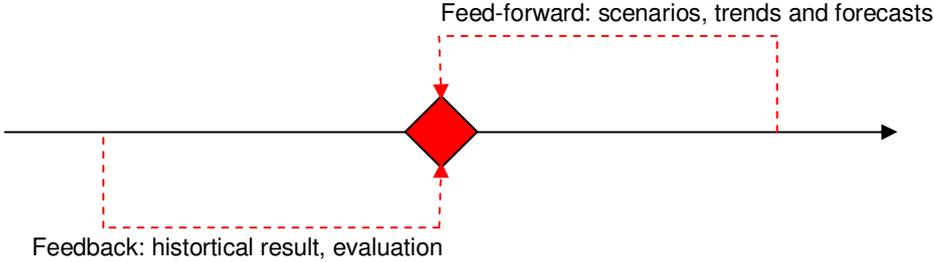
Figure 2.3 Feed-forward and Feedback system
