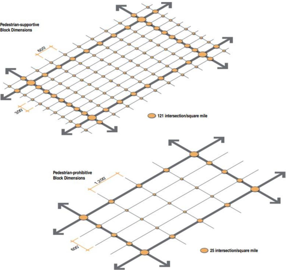
Figure 3. Options for scaling and designing blocks and road frontages. (Source: Pace, 2013.)
