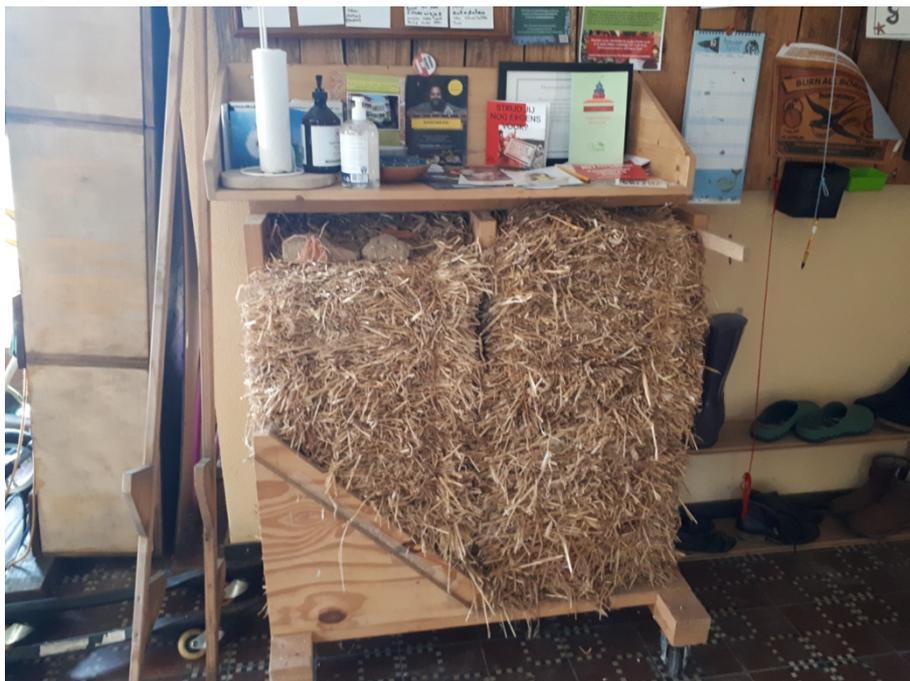
**Figure 10:** A sample of a straw building block used during the construction of the IEWAN apartment complex and showed during the monthly educative tours.
