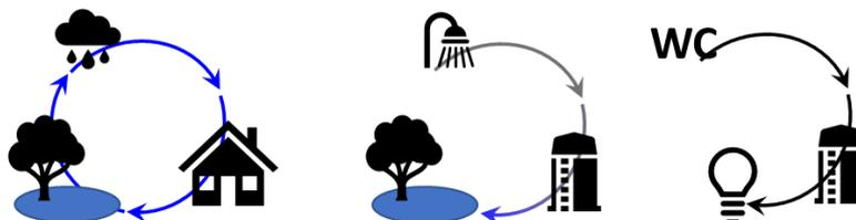
Figure 9: Principle of the Hamburg Water Cycle, from left to right: Rainwater, greywater and blackwater (modified after Hamburg Wasser, 2017).
