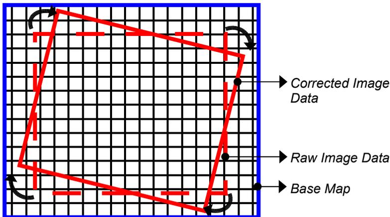
Figure 3.2 Geometric image corection process. (Sardana, 2005)
